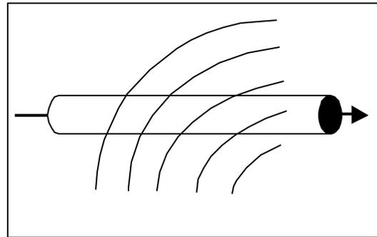
Figure 3 – Current Flow Resulting From Induced Voltage
