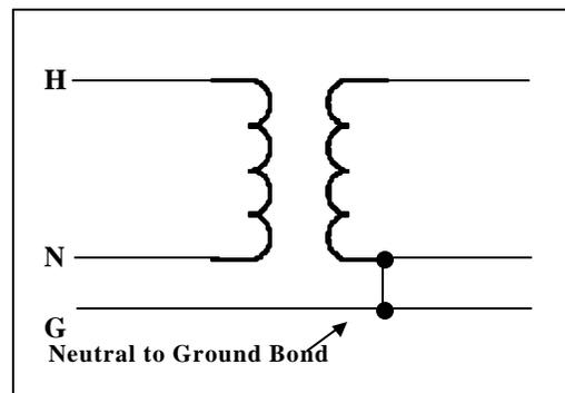
Figure 4 – Output Neutral to Ground **Bond**
