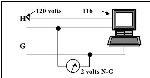
Figure 2 – Voltage Drop at Long Branch Receptacle
