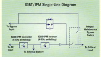
TOP: An on-line doubleconversion system configuration for an IGBT/IPM, including a transistorized converter and inverter.
