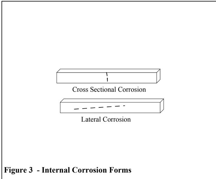
cross sectional fault will exhibit a high impedance quicker than the lower representation. The lower, lateral corrosion example will mask the increase in impedance by generating a parallel current path until a full fracture occurs. Figure 4 shows the impedance life of a particular VRLA cell which failed due to negative bus strap corrosion. From October 27, 1994 until February 16, 1995 the impedance
