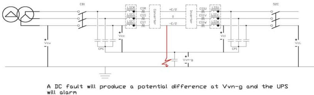
**Figure 13: DC Ground Fault**
