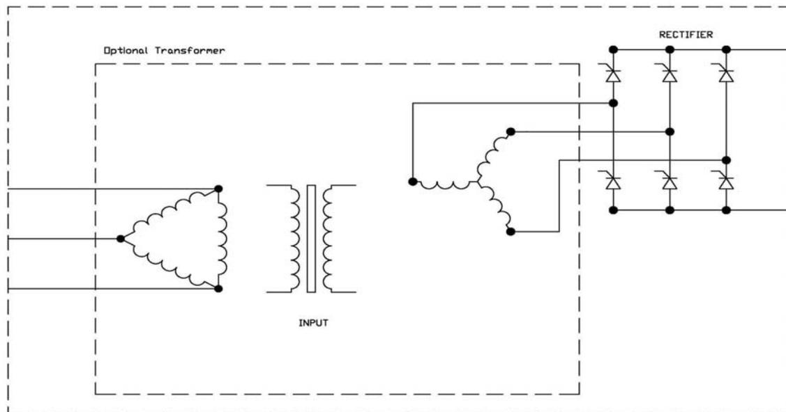
**Figure 1: 6 pulse rectifier with optional transformer**
