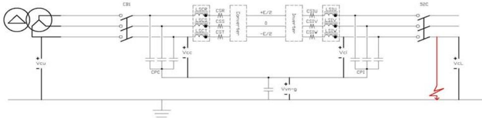
A Phase to Ground fault when the upstream transformer is not grounded will produce a potential difference at  $V_{vn-g}$  and the UPS will alarm
