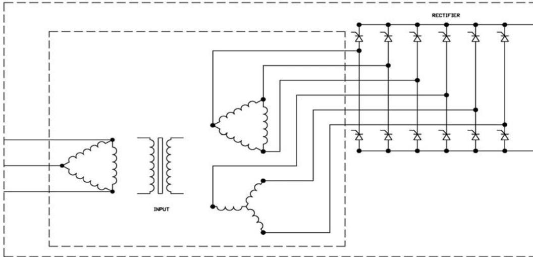
**Figure 2: 12 pulse rectifier with optional transformer**
