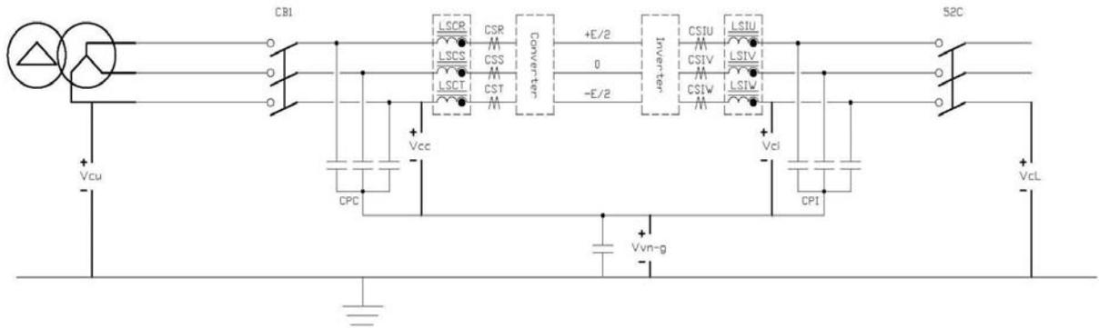
The voltage  $V_{vn-g}$  is monitored and will be approximately zero
