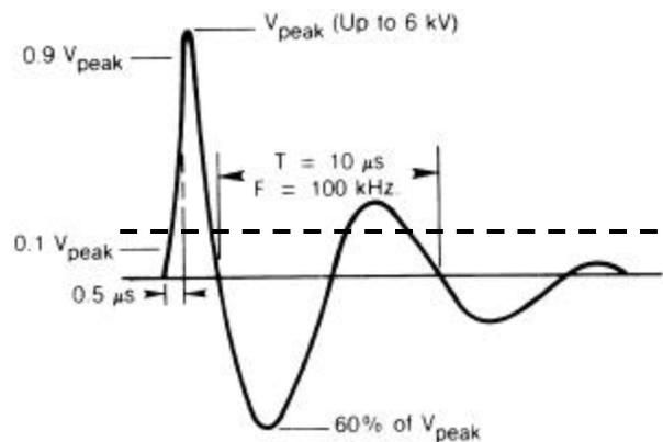
Obviously, the lower a TVSS unit can clamp the transient voltage, the better it can protect the connected equipment. What you may not know, however, is that 300 volts or so is about the best that any TVSS unit can perform, and it isn't that difficult or expensive to build a TVSS that can do that kind of job. In addition, most TVSS technologies share a great deal in common, particularly with regard to the types of components that are used. And that's where the story gets interesting.
